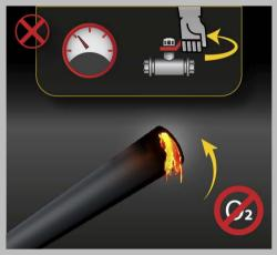
DO NOT EXTINGUISH THE LANCE TILTING IT UPWARDS.
