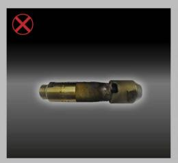
7) DO NOT USE THE LANCE HOLDER IN CLEARLY BAD CONDITIONS, WITHOUT MAINTENANCE OR WITH OXYGEN LEAKAGE.
