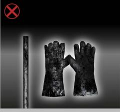
DO NOT USE CONTAMINATED PPE DURING LANCING OPERATION WITH COMBUSTIBLE OR ORGANIC MATERIALS (FUEL, OIL, GREASE, OTHERS).
