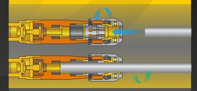
After checking that everything - oxygen network, personal protection equipment and work area - is in perfect condition, insert the lance fully into the the lance holder, tighten thoroughly with the locking nut and check that there are no leaks.
