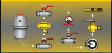
For the operation of thermal lances we recommend to have a standard oxygen line, (with seals, shut off and regulating valves and filters) that supply oxygen with not contaminants.
