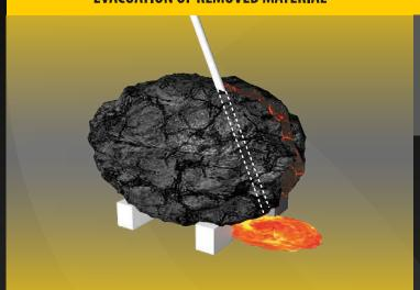
Cuts are preferably made from top to bottom as the molten material requires to be evacuated from the channel, or it will be solidified again when cools down affecting the achieved progress. Therefore, it is necessary to make a molten material evacuation channel. **The bottom of the material to be cut should not touch the ground.**
