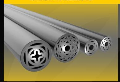
The greater the thickness of the object to be cut, the greater diameter the thermal lance diameter. As long as it corresponds to the same type of thermal lance. With this way, it is possible to evacuate the molten material easily through the cutting channel made by the lance, without the risk that molten material solidifies. It also reduces the risk of lance jamming.
