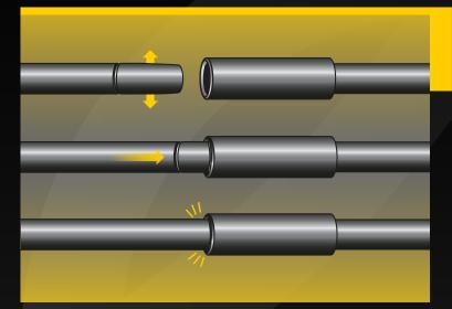
1) Align the tip of the used lance with the new lance connector. Gently insert the part of the used lance until you feel a "click", now they are tightly connected. Always check the connection by trying to pull it apart or backwards.
