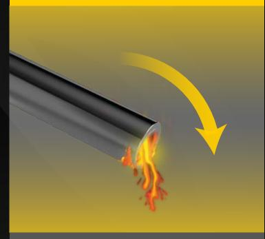
Incline the lance with the tip down to make it easier for the melted material to come off the thermal lance.
