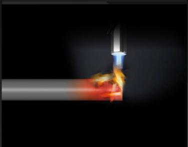
This type of ignition is performed using external heat sources for heating the tip of the lance, such as: torches, oxyfuel, electric arc, hot materials, etc.
