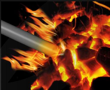
This type of ignition is made with combustible materials such as coke carbon, wood, cardboard, etc., taking advantage of oxygen to accelerate combustion. To ignite the lance with this system, the tip of the lance should touch the combustible material and allow a low amount of oxygen to pass.
