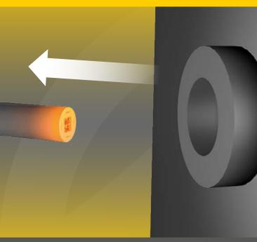
Remove the thermal lance from the object. NEVER CUT THE OXYGEN FLOW WHILE THE LANCE IS STILL IN CONTACT WITH THE MELTED MATERIAL.
