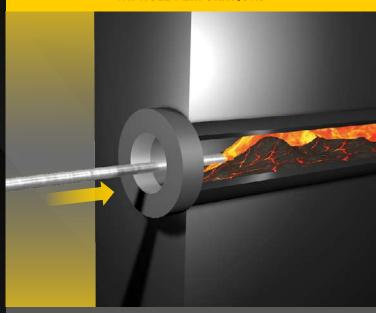
1) When the flow of material trough the passage is reduced by any obstruction of solid material or loss of fluidity by cooled metal, insert the lance until it touches the hard material and push with a gentle yet steady pressure advancing as it perforates the obstacle.
