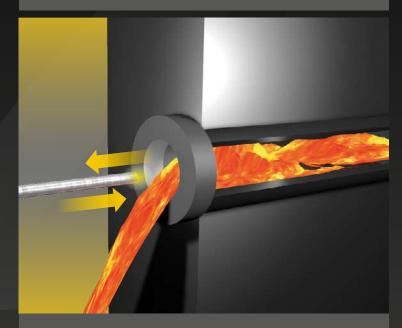
2) If the lance passes through the obstruction and the flow remains low, re-insert the lance until it touches the obstruction and repeat the operation with swaying movements until clearing the passage.
