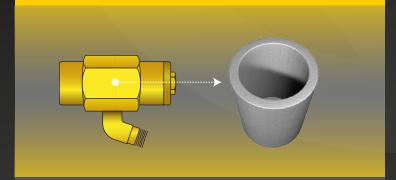
A filter of at least 40  $\mu$ m (microns) must be provided at each oxygen connection point to avoid the arrival of particles that can generate temperatures in the hose with risk of ignition.
