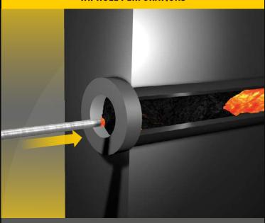
1) The lance is introduced into the taphole until it passes through the mud plug and reaches the liquid material to be evacuated. To perform this operation, place the ignited tip of the lance against the center point of the passage by pressing gently, avoiding to separate from the material to be perforated.
