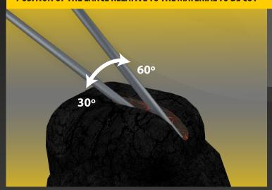
The lance must always attack the material to be cutted with an inclination between 30  $^{\circ}$  and 60  $^{\circ}$ , and the operator defines the better inclination.
