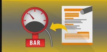
For efficient use of the lance, it is key to regulate the specific oxygen flow for each type (according to the technical sheet). We recommend having a pressure gauge in the socket for the lance. If connected to an oxygen tank, use a high flow regulator.
