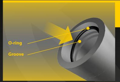
2) If the connector does not fit in easily, do not apply force. Disconnect and check for any foreing material or if the O'Ring has been removed from its slot. In that case, just relocate it by moving it into the groove with your finger.
