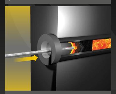
2) Maintain a gentle pressure all the way until you perforate the taphole. Do not make lateral movements with the lance, unless it requires a conical perforation or if you are not using the proper diameter of the lance. Then, it must be removed and placed in different points of the mud plug until achieving the desired perforation.
