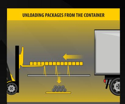
After unpacking the packages from the container, unload one by one by placing 2 or 3 slings, verifying that they are balanced when being lifted.
